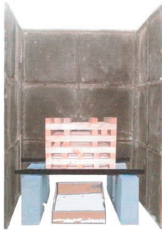
Figure 6 Wood crib ignition arrangement
