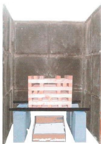
Figure 6 Wood crib ignition arrangement
